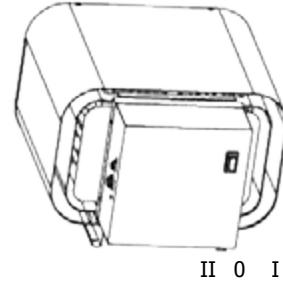
In case of breakdown, press the control unit switch on the left part of the rocker to the middle position (switch position 0). The unit is now completely switched off.
